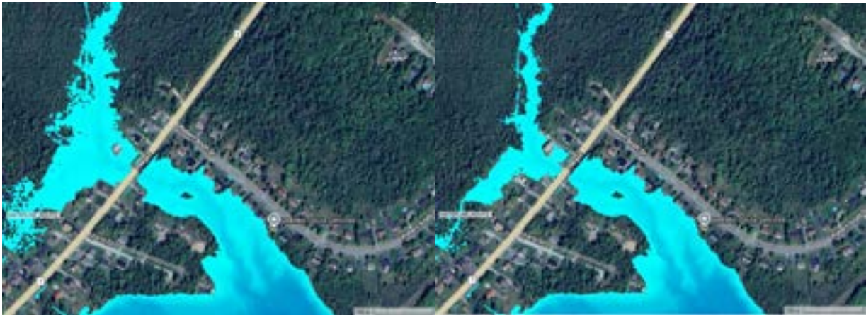
Figure 16: Highway 2 near Robert Scott Drive with twin 2,400mm upgrade (existing condition left, proposed recommendations right)– 1% AEP (Existing)
