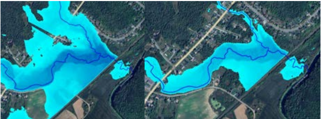
Figure 15: Outlet of the system with triple barrel upgrade (existing condition left, proposed recommendations right)– 1% AEP (2100)
