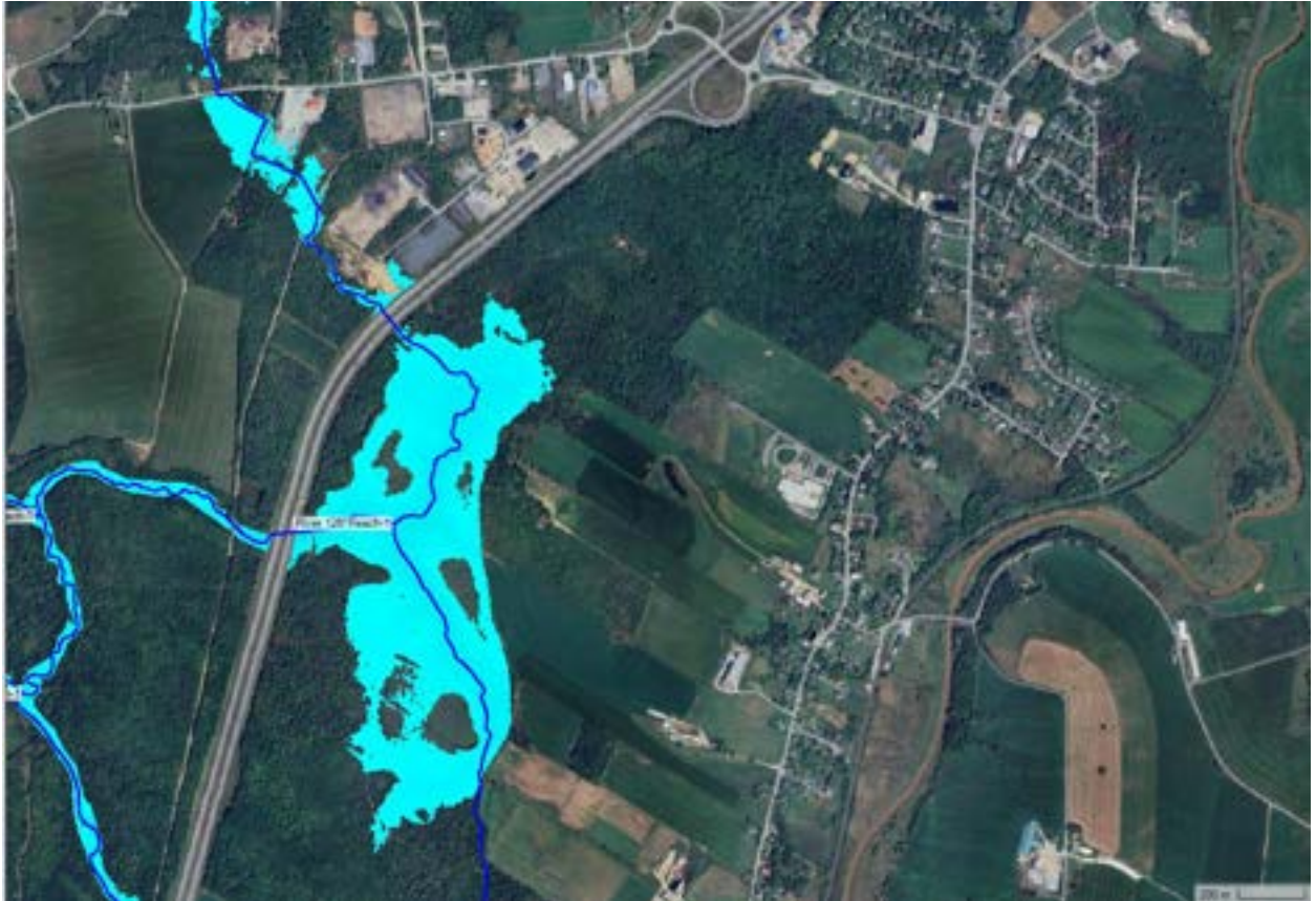
Figure 13: Highway 102 Flood Extent - 1% AEP Existing
