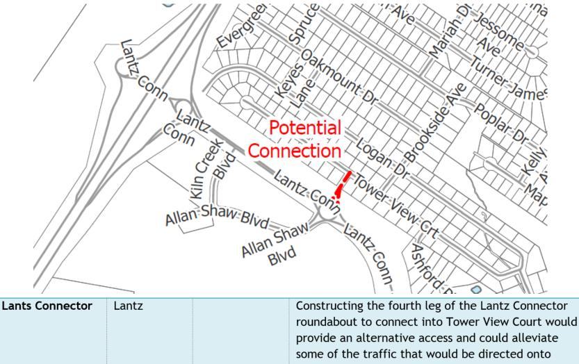
some of the traffic that would be directed onto Highway 2 in case of emergency. The roundabout connection to Tower View has many other benefits to the community as well.
