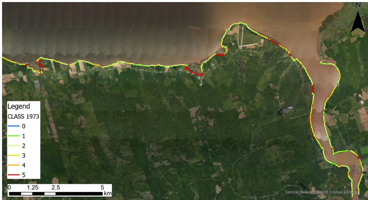
Figure 6. Classified erosion rates from the Shubenacadie River to Noel Shore, NS.
