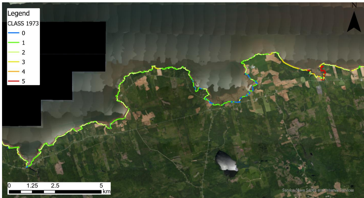
Figure 7. Classified erosion rates for the Noel Shore to Moose Brook, NS.
