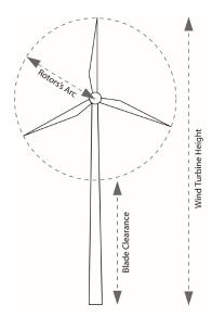
**Wind Energy, Blade Clearance** means the distance from grade to the bottom of the rotor's arc.
