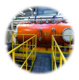
Feedstock is roasted at high temperatures in the absence of oxygen (pyrolysis) to produce a stable carbon product
