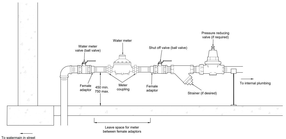
5/8" water meter - 12" space, 3/4" female adaptor 3/4" water meter - 13 3/4" space, 3/4" female adaptor 1" water meter - 15 3/4" space - 1" female adaptor
