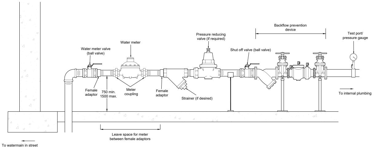
5/8" water meter - 12" space, 3/4" female adaptor 3/4" water meter - 13 3/4" space, 3/4" female adaptor 1" water meter - 15 3/4" space - 1" female adaptor
