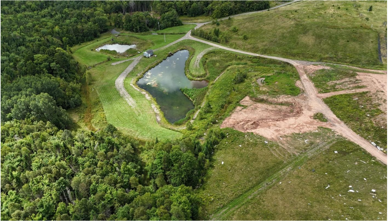
Ph 5 - Existing Sedimentation Control Ponds
