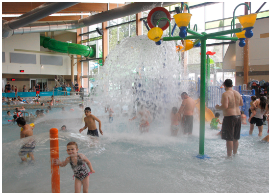
Kinetic water features on a fixed pipe grid allows elements to be moved around or replaced over time to maintain the novelty factor
